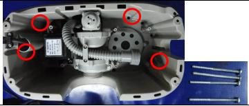
$2\sqrt{1000}$  Loosen four screws (ST4\*60) from the bottom of the cabinet
