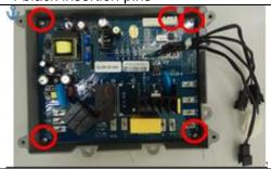
7. Loosen the fixed screws on circuit board; Take out the circuit board; Remove the tie and insertion between Circuit board and data cable.
