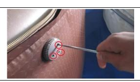
2. Unscrew the screws of the air valve.;
