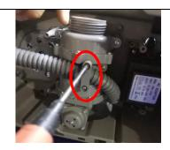
5. Take out the metal tube in the air tube with a screwdriver
