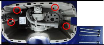
2. Loosen four screws (ST4\*60) from the bottom of the cabinet
