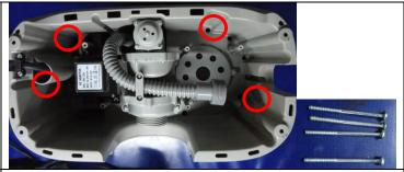
2. Loosen four screws(ST4\*60) from the bottom of the
