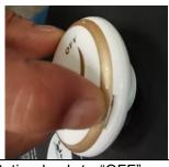
1. Turn the rotation knob to "OFF" position, open and remove the top cover by hand(as shown in photo)
