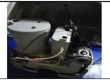
3. Loosen five screws (ST4\*15) from the rear cover of the cabinet; Loosen two screws (ST4\*15) from the base of the cabinet
