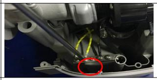
10  $\,$  Use cross screwdriver to disassemble the 2 heating earth wire
