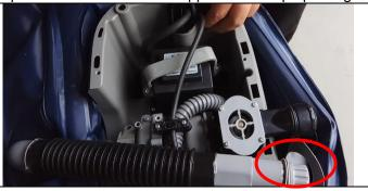
3. Remove the fixed ring of the water drainage assembly;
