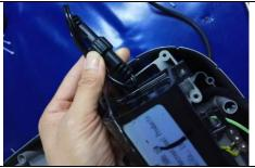
8. Take down the filter pump; Loosen the signal cable between filter pump and transformer; Assemble the new filter pump into the control box in reverse order. (Video available)
