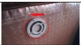
3. Unscrew the nut of the air valve.;
