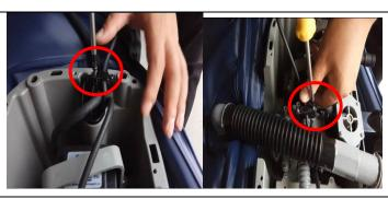
4.1. Remove the fixed pressure plate of JET power cord; (For Elite series only, video available: How to disconnect Jet cable before taking out control box)
