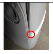
3. Loosen five screws (ST4\*15) from the rear cover of the cabinet; Loosen two screws (ST4\*15) from the bottom of the cabinet
