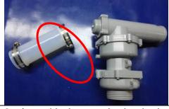
Take out the check valve, remove the metal tube in the other end.
