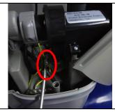
7. Use a screwdriver to remove the metal clamp in the connection between the filter pump and the water pipe;
