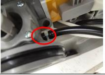
9. Remove the binding band of the O3 inlet pipe on the PTC assembly and remove the O3 inlet pipe;
