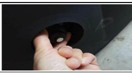
4. Remove the manometer cap and release the air of liner;
