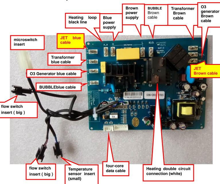
Elite series with JET brown cable and jet blue cable connected Premium series without JET brown cable and jet blue cable due to no Jet function
