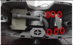
9. Loosen 2 screws from transformer support; Then loosen the 4 screws and take out the original transformer. Assemble the new transformer into the control box in reverse order.
