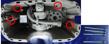
2. Loosen four screws (ST4\*60) from the bottom of the cabinet
