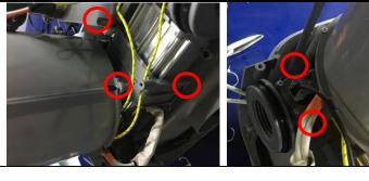
7. Loosen 6 screws from the filter pump
