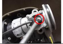
5. Loosen the fixed screws and take out old reed switch; Assemble new reed switch into the control box. If replace the reed switch from heater element, need to remove the bubble generator and reed switch first.
