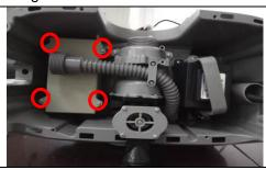
7、Remove the connection strap of the O3 joint pipe and the one-way valve with inclined tongs, and remove the O3 joint pipe;
