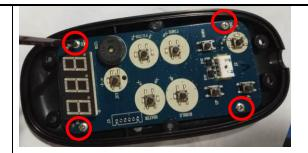
3. Take down the data cable and Transparent buttons (8 buttons for Premium/Concept version, 9 buttons for Elite version)
