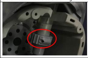
4.2. Disconnect two pairs of JET inserts from JET cable insertion hole ( For Elite series only )
