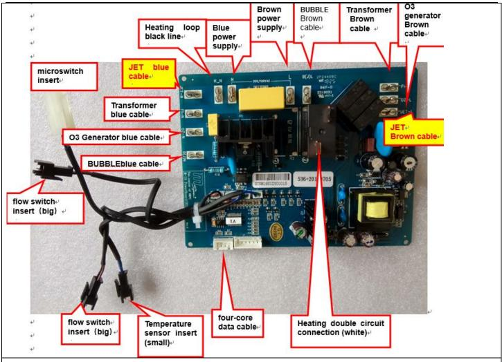
8. Assemble the new power board into the control box in reverse order. (Video available)
