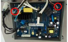
5. Loosen three screws from the fixed junction box; disassemble 4 sets black pin-cable;
