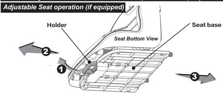
Lifting up the holder inside the seat while moving the seat forward and backward.
