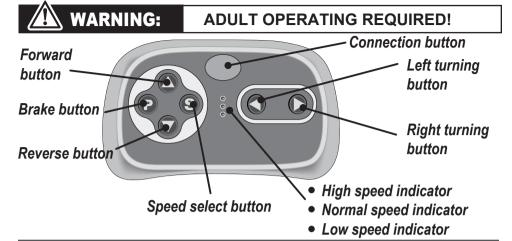
The remote control has precedence over foot pedal operation. (The foot pedal won't work while you operate the Remote Controller)
