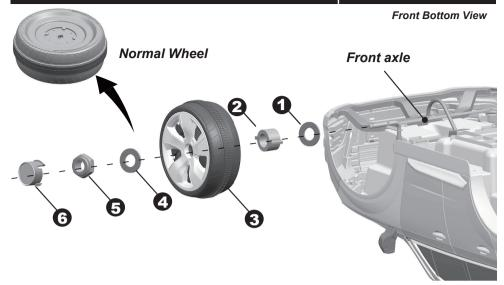
Remove all the parts from the front axle.
