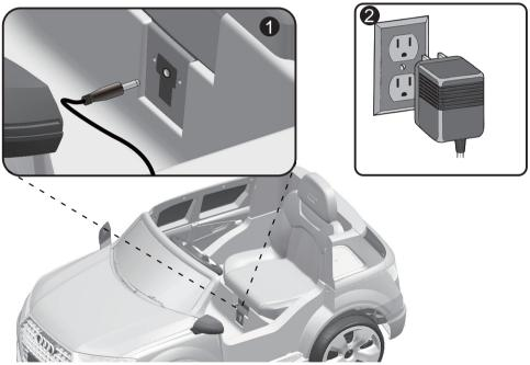
1. Plug the charger port into the input socket. (the socket is below the seat) HINT: If your vehicle equipped with the Multi-function Dash, the Charging Socket is on the dash, please see page 17 <Use the Multi-function Dash> 2. Plug the charger plug into a wall outlet. The battery will begin charging.
