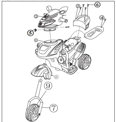
Instruction: (1) car body (2) head components (3) backrest (4) toolbox (5) nut (6) rearview mirror (7) hubcap (8) lock (9) wheel
