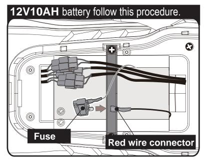
• Locate the red wire connector and plug it into the terminal on battery.
