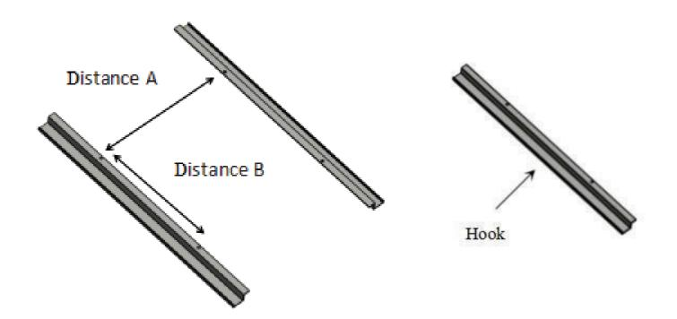
2. Mount the two hanging units onto ceiling with screws, and turn the screws to the end tightly, this is very important.
