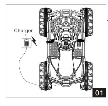
1. Battery charging: (see figure 01) When the battery is insufficient, please promptly to the battery. The charging jack on the car is behind the center location. (note: toys not operating charging condition. Charge should be charged under adult supervision) rechargeable batteries should be removed from the toy.
