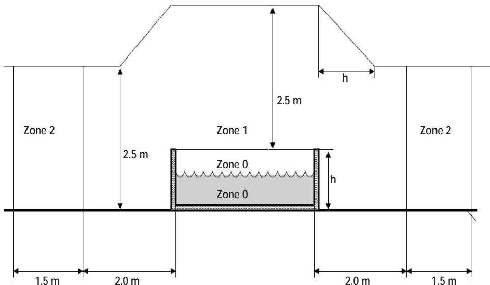
**NOTE-**The measured zone dimensions are limited by walls and fixed partitions.
